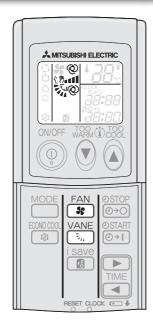
Press to select fan speed. Each press changes fan speed in the following order:
