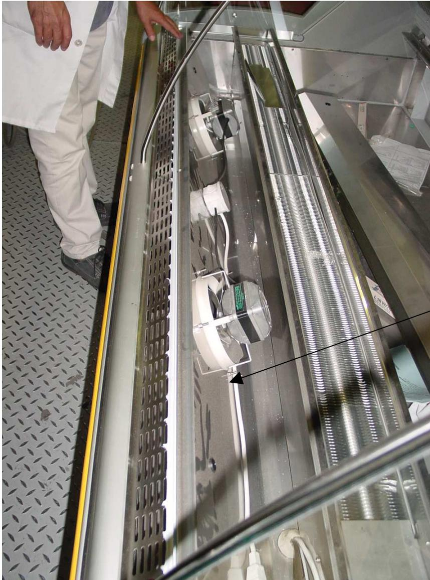
7) Place correctly the ventilators heads
