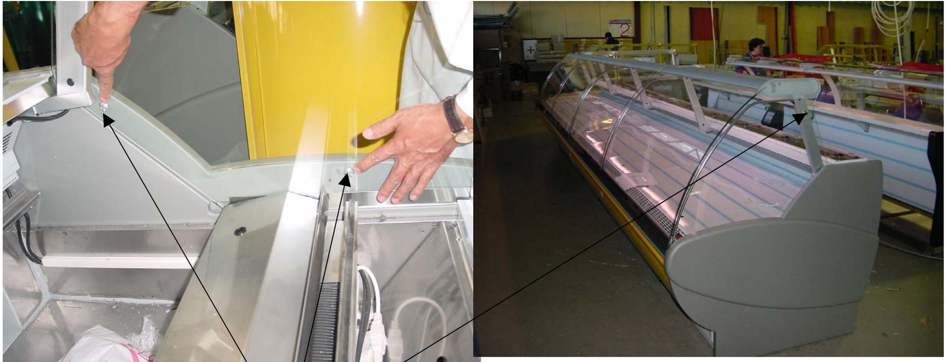
**19)** At last, you need to put the side glass as shown. Then screw it on the upper structure, but do it by the outside (aluminium support).
