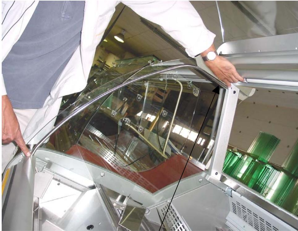
**12)** Place the tube that supports the structure in the front and upper gadgets as shown.
