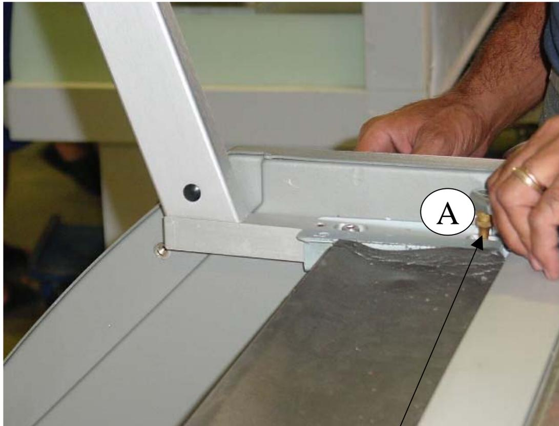
**14)** Screw completely (A) with key Umbrako n° 6, and put the aluminium support as shown.
