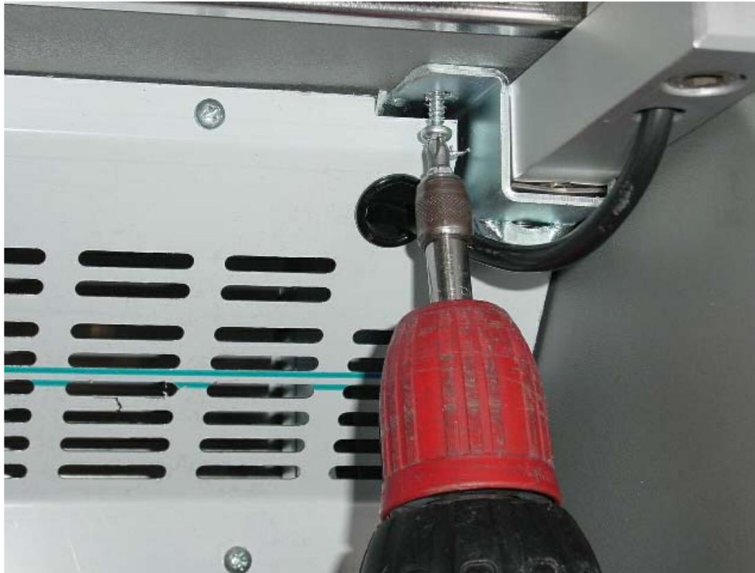
**17)** To fix the service plate, you'll have to screw by the exhibition part, the necessary points ( 2 or 3 in accordance the the cabinet width).
