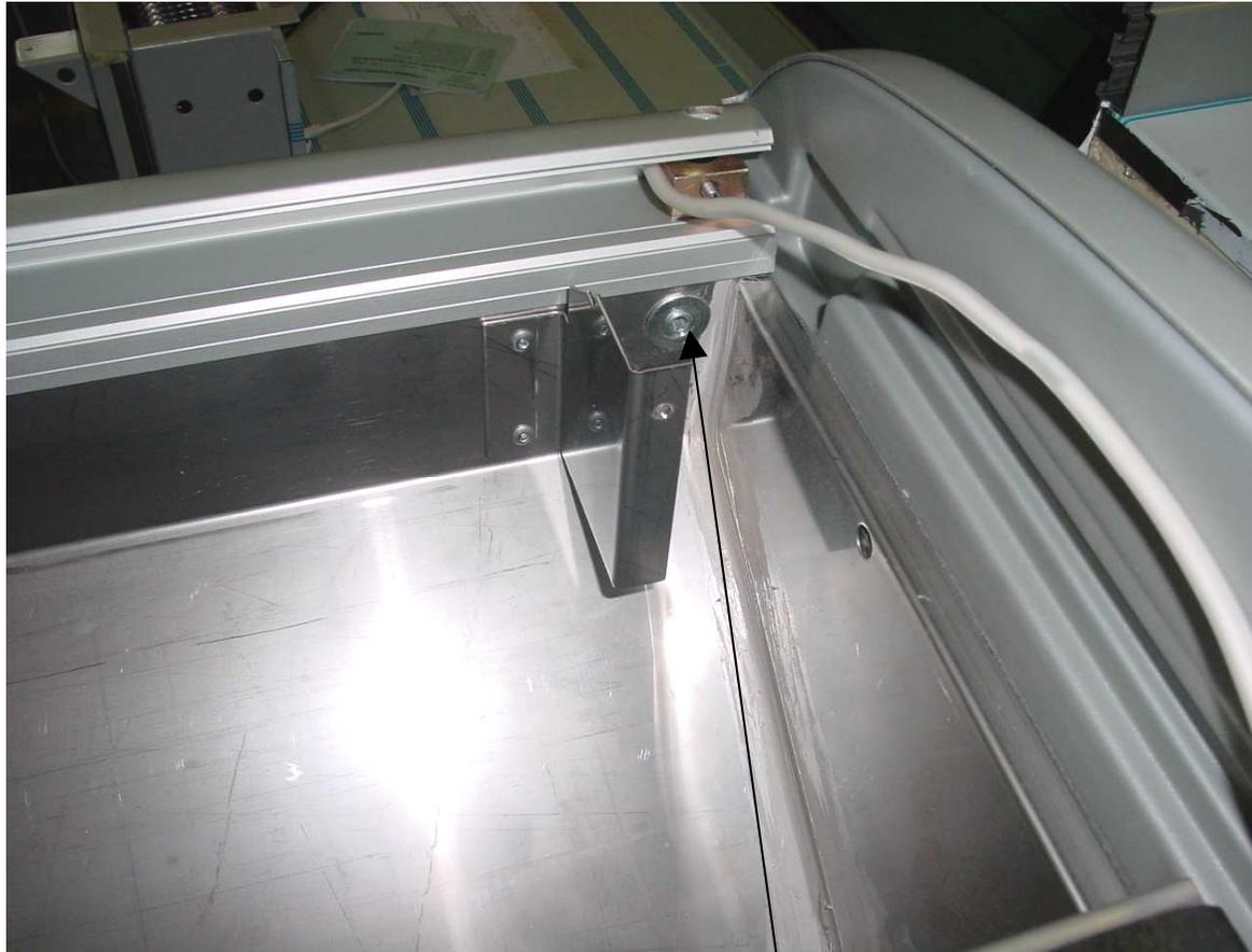
**2)** Screw with « Umbrako » N°.5 to assemble including the side part.
