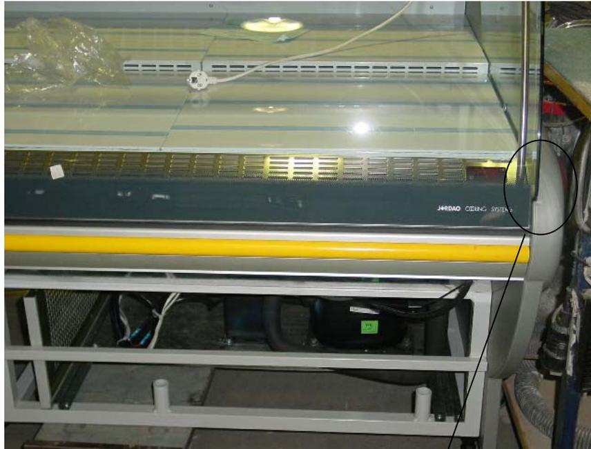
**A)** Between the front structure and the side part it shall have 2 or 3 mm.
