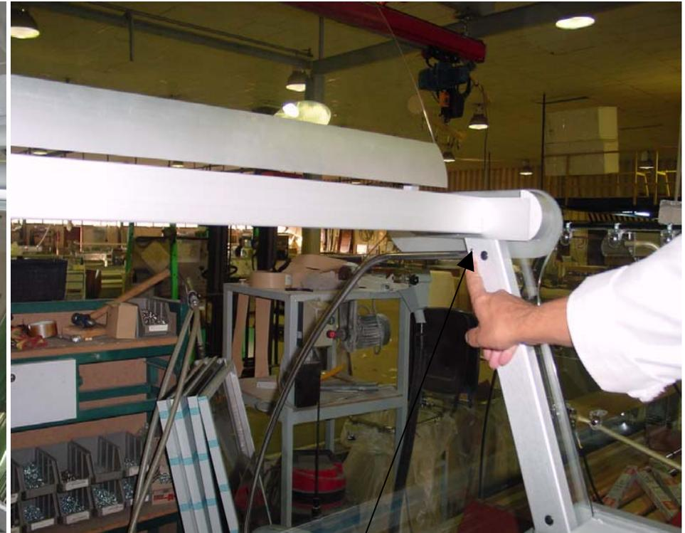
**13)** Screw with key Umbrako N°.3 in the position shown in the picture, to assemble the tube.
