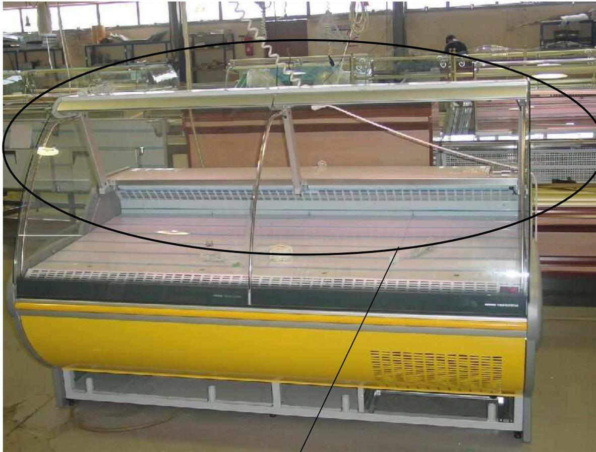
**11)** If the cabinet arrives without the glasses assembled, you need to place the aluminium supports structure, which is sent all assembled.
