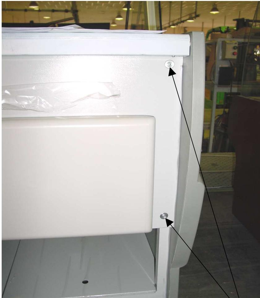
**4)** Screw with key « Umbrako » N°.5 to assemble these parts
