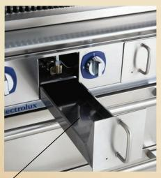
Large removable ½ gal. (2 l) grease collection drawer, full depth of charbroiler (one per burner); can be filled with water to aid cleaning
