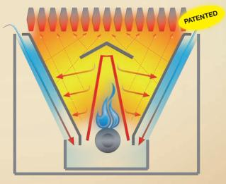
• Highly efficient heating system: the flame heats the radiant shield bringing the temperature above 1290°F (700°C). The heat is then radiated towards the heat deflectors and onto the cooking grate, thus guaranteeing an even temperature throughout for excellent grilling results across the entire cooking surface
