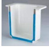
ColdFest Food Pans are made with high-impact resistant ABS shells and non-toxic refrigerant gel cores.
