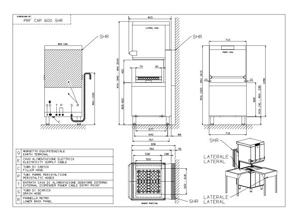
\* Indicative wash times \*Cold water connection required and three-phase electrical connection whenever possible
