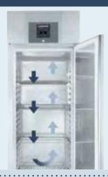
**Air ducting system for excellent temperature distribution.** The innovative air ducting system is designed to maintain freshness during food storage: two fans draw the air over the cooling evaporator, then it is directed downwards behind an air deflector. This ensures constant air circulation – and uniform temperature distribution.
