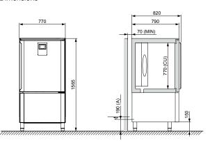
(M1) MX45ATS (A) Electrical supply (CU) Useful (MIN) Minimum
