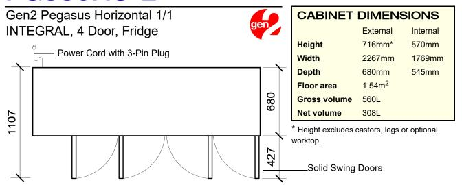
Electronic Side Mounted Integral Refrigeration Unit
