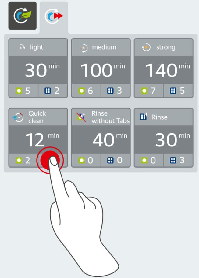
Quick cleaning easily found and quickly activated. Simply place the cleaner tabs in the drain strainer and start the clean. Production can then resume after no more than 12 minutes.
