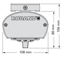
Dimensions for fabricator infra-red heating assemblies (HUE models). Brackets are removable.
