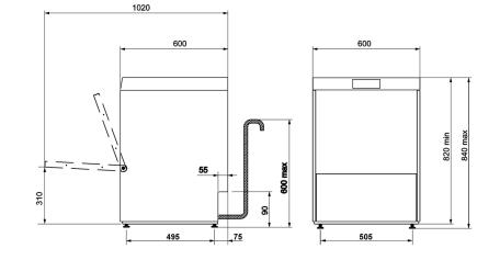
\*Supplied water temperature >50°C and <60°C and three-phase electrical connection whenever possible. \*Indicative wash times
