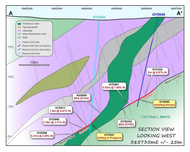
Figure 5: Goodyear Cross section (385735mE) Looking West
