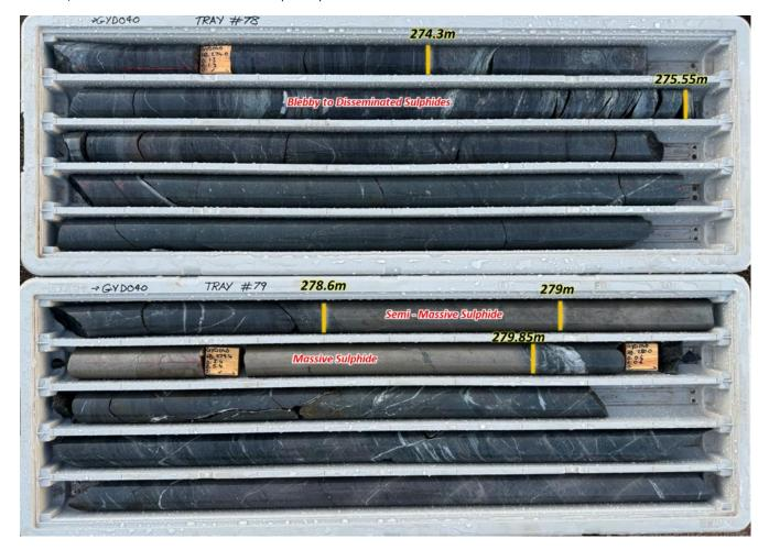
Figure 4: Sulphide intersection within GYD040
