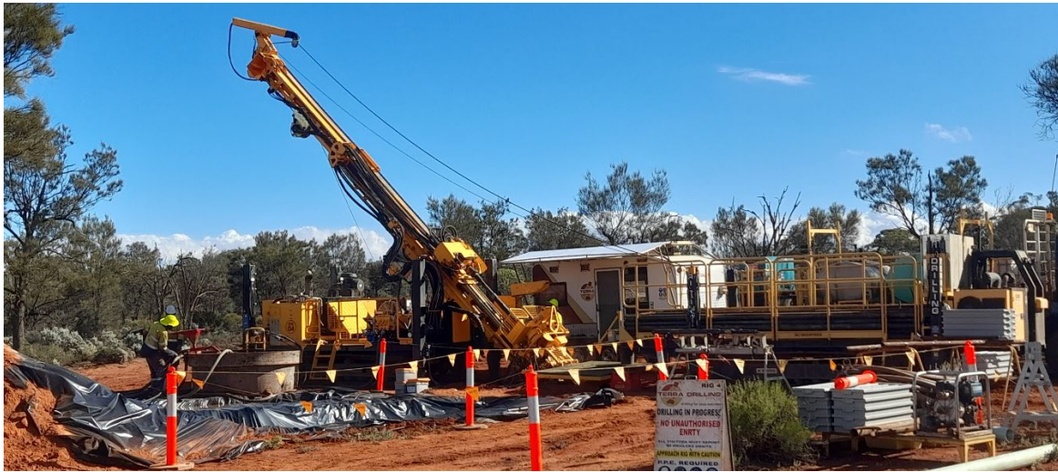
Figure 5: Diamond Drill Rig in support of a potential Stage 2 open pit at Lucky Strike.
