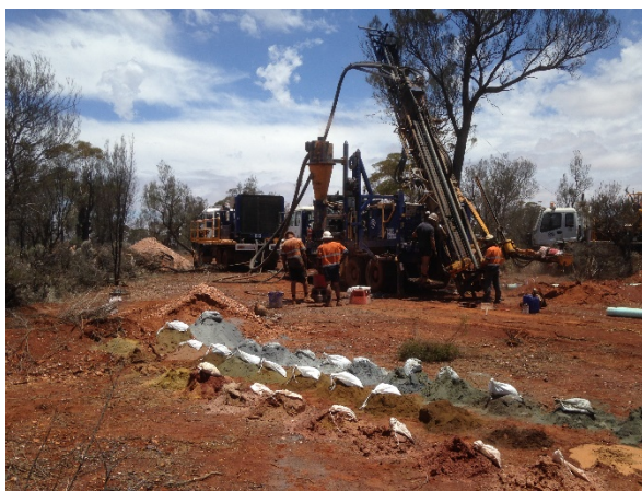
RC drilling at Lucky Strike January 2018 (Hole LEFR028-looking south west)
