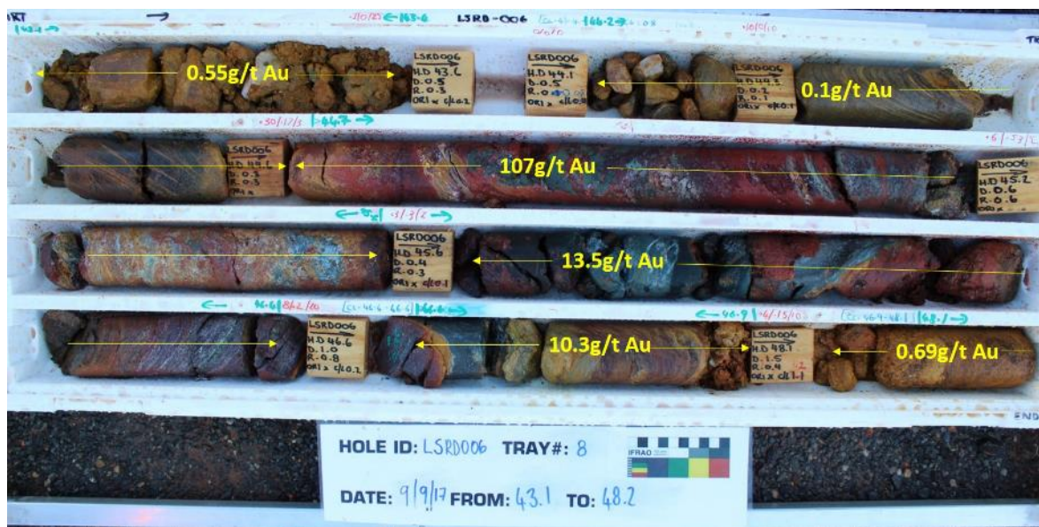
Figure 4 Core tray from Hole LSRD006 displaying highly oxidised BIF and high grade gold intersections (Core tray interval 43.1-48.2m)
