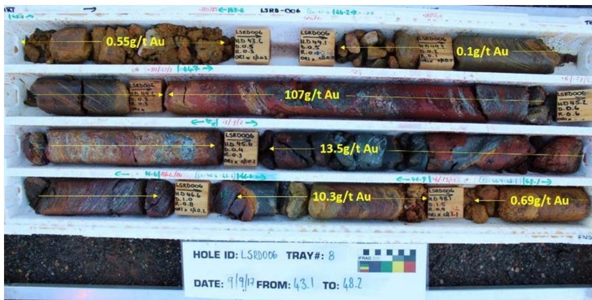
Figure 5 Core tray from Hole LSRD006 displaying highly oxidised BIF and high grade gold intersections (Core tray interval 43.1-48.2m)
