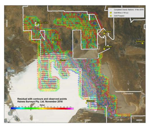
**Figure 2** Inset map showing preliminary residual gravity image and completed gravity stations within and near Lake Lefroy
