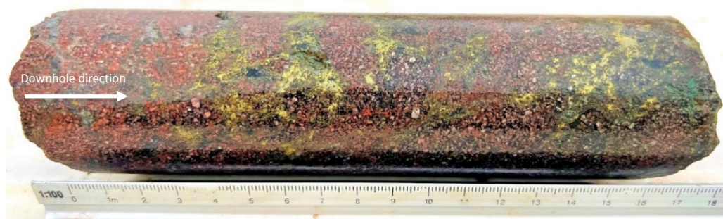
LEFD006 Hematite altered porphyry with chalcopyrite 0.5g/t Au and 2.3% Cu. Refer Figure 3 for detail
