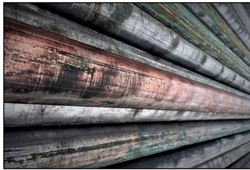
Copper coated drill rod from LEFD008
