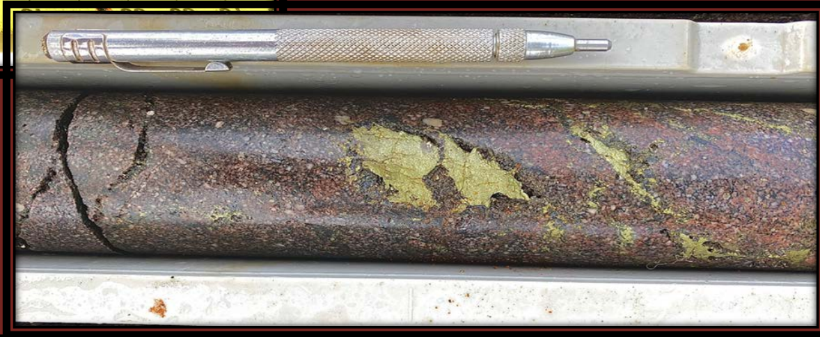
LEFRD267 interval 301 – 301.3m showing chalcopyrite in association with a gypsum magnesite vein in basalt. (9.92g/t Au and 2.3% Cu). Gypsum vein contains visible gold.
