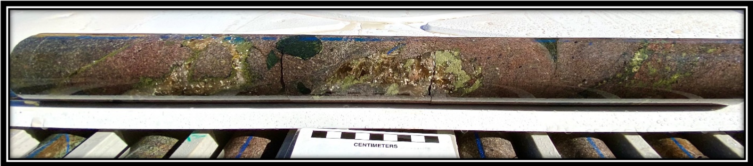
Figure 7 LEFRD267 interval 311 – 311.5m showing chalcopyrite with anhydrite, magnesite and strong hematite (red) alteration in quartz feldspar porphyry. The interval also contains a mafic xenolith
