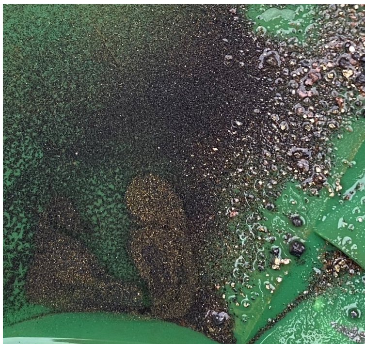
Figure 4 Fine gold panned from interval 148-149m in LEFR260 (black material is magnetite)
