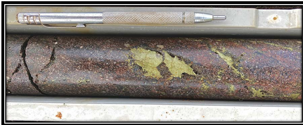
Figure 7 OBURCD025 --231.37m-231.6m diorite porphyry- blebby chalcopyrite (4.61g/t Au & 1.1% Cu)
