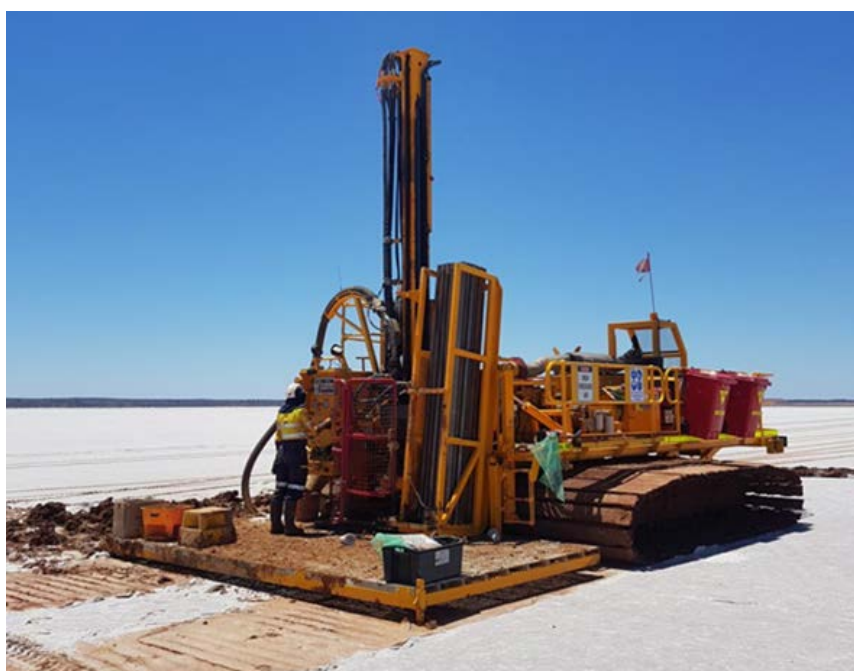
Figure 3 Specialised lake aircore drill rig on Lake Lefroy (Photo courtesy of Gold Fields)
