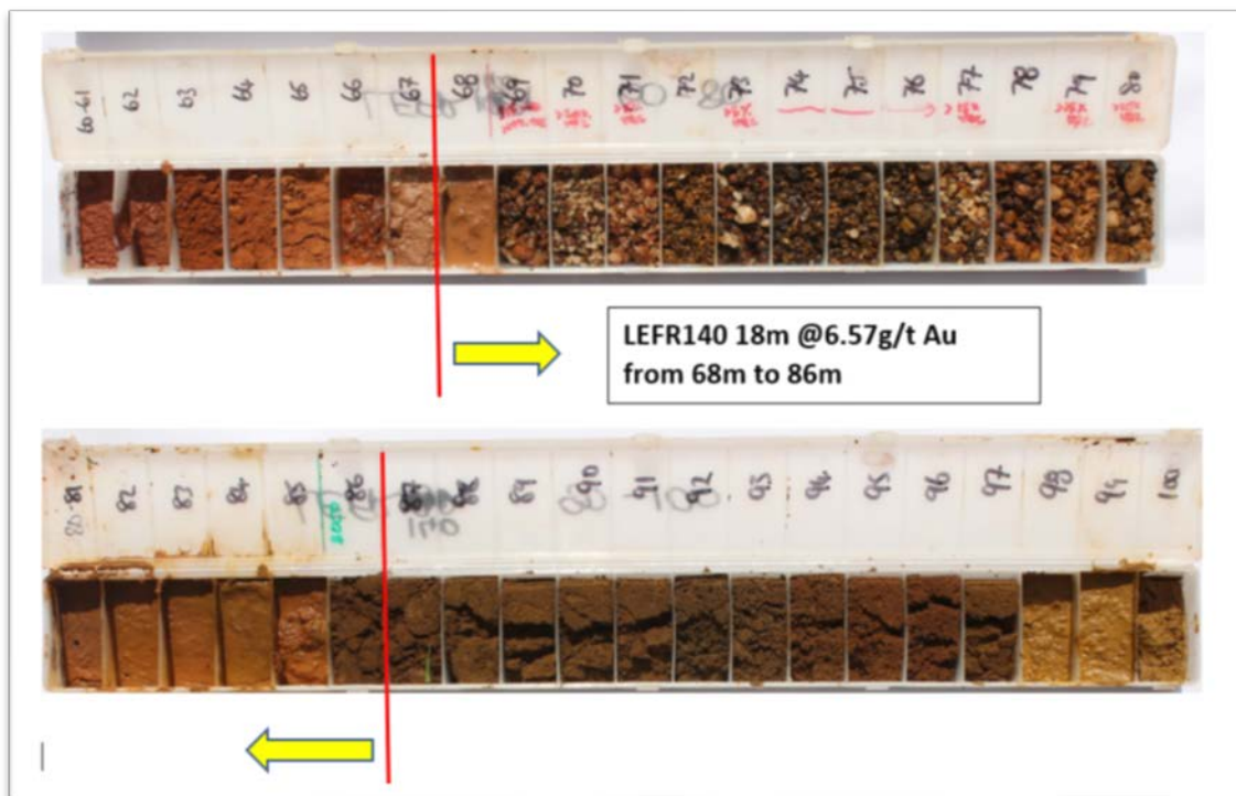
Figure 5 RC Drill chips from LEFR140 displaying the oxidised strongly gold mineralised BIF interval. Each compartment represents a 1m downhole consecutive drill interval.
