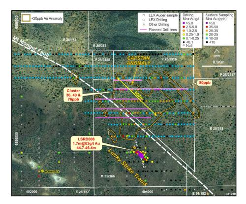
Figure 2 Capstan auger gold anomaly sample points and proposed drill lines with proximity to Lucky Strike.
