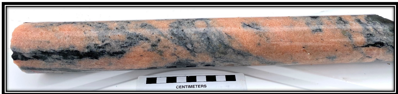
Figure 7 LEFRD261 339-339.4m (Lower basalt) showing pink calcite vein with chalcopyrite and pyrite blebs from within a basalt host rock (339m-340m 0.28g/t Au, 0.01% Cu, 192ppm W)
