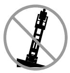
Do not depend on the tilt alarm as a level indicator. The tilt alarm sounds on the chassis only when the machine is on a severe slope.
