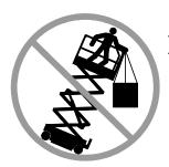
Do not place or attach fixed or overhanging loads to any part of this machine. Do not transport tools and materials unless they are evenly distributed and can be safely handled by person(s) in the platform.
