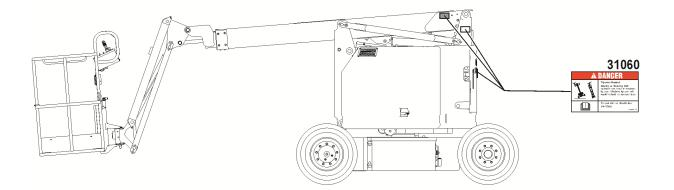
\*\* These decals are installed on both sides of chassis.
