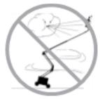
Do not raise the boom when wind speeds may exceed 12.5 m/s. If wind speeds exceed 12.5 m/s when the boom is raised, lower the boom and do not continue to operate the machine.
