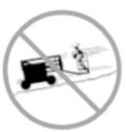
Limit travel speed according to the condition of the ground surface, congestion, slope, location of personnel, and any other factors which may cause collision.
