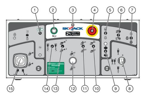
Figure 2-7. Platform Control Console
