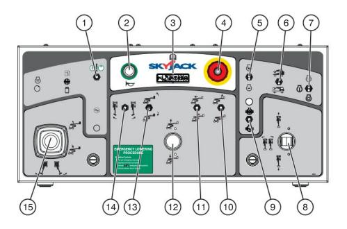
Figure 2-7. Platform Control Console
