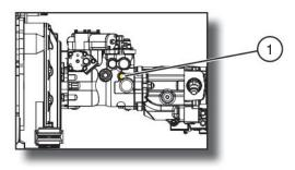
Figure 2-2. Drive Bypass Valve
