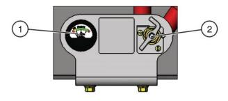
Figure 2-1. Main Power Disconnect Switch & Battery Charge Indicator
