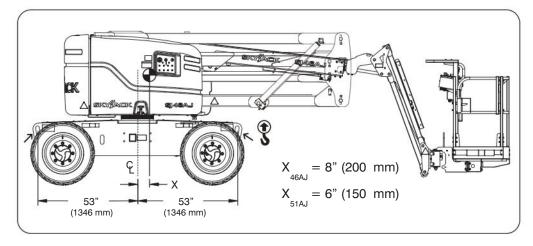
Figure 2-11. Lifting Points NOTE: Center of gravity varies with different options.
