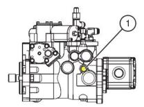
Figure 2-12. Drive Bypass Valve
