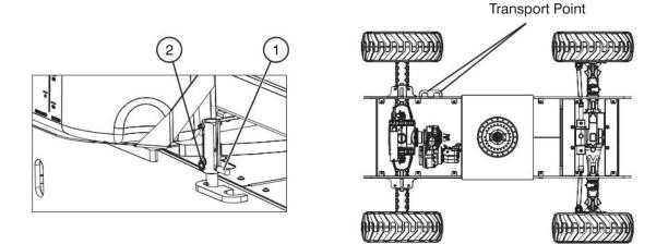
Figure 2-10. Turret Transportation Lock & Locking Points
