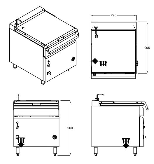
**W** 415/240V N+E 50Hz 1/2" Quick Connect Water Inlet
