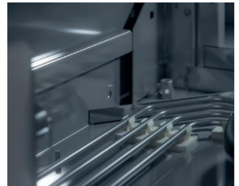
The two-part\* rack holder is easy to remove, enabling easy access for cleaning.
