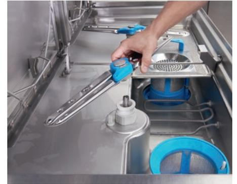
The blue operating concept: any parts that are blue can be removed, washed and replaced. The *M-iClean H* automatically checks that everything has been put back in the right place.
