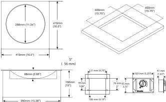
The CookTek® Drop-in Induction Wok with Standard Controls boasts a drop-in countertop design with a stainless steel top, aluminum housing, and a recessed glass- ceramic wok bowl intended for commercial kitchens and restaurants. An automatic shut-off feature, integral cooling fan, and self-diagnosing microprocessor allow for a safe kitchen environment. Each unit is equipped with 20 precise power settings to ensure maximum and efficient heating of any induction compatible wok pan.\*
