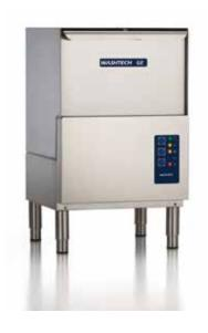
The unit shall be a Washtech glasswasher with Watermark certification. The glasswasher shall have a one minute complete operating cycle including operator selectable cold final rinse. The unit shall accept racks 365mm x 435mm square with 290mm door clearance for tall glasses. A detergent injector shall be fitted and the unit shall be supplied in 100% recyclable shipping packaging. Electrical supply to be 15 amp single phase.
