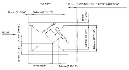
NOTE: IF THE UNIT IS INSTALLED AS A BUILT-IN/UNDERCOUNTER, BETWEEN 5 AND 10 mm ON EACH SIDE MUST BE CONSIDERED TO ALLOW FOR EASE OF INSTALLATION
